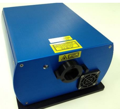
Typical Open Beam MOPA Profile
